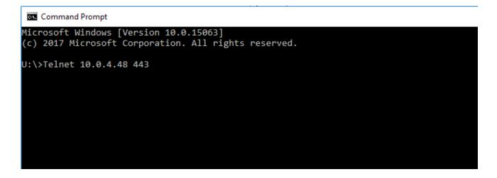
If the device can successfully connect to the Name & Connectivity Server port, the command prompt window will go blank.
